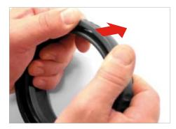
Press the Lock and Release Ring backwards with your thumbs until you can access the O-ring. **NOTE:** Do not use excessive force as that might break the rings.
