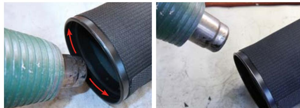
Start by heating the inside of the ring. Move the nozzle of the heat gun constantly, as displayed by the red arrows, to prevent the ring and suit from overheating. The next step is to heat the outside of the drysuit in order to get a smooth and constant melting point of the adhesive.
