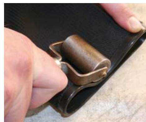
When the adhesive has melted and the ring is in place you need to squeeze away all air-pockets in order to get maximum grip between the components. Use a roller or similar tool to put equal force over the actual surface. Roll back and forth until you have covered the complete surface 360°. When this is done we recommend you to wait about 10 minutes before starting the next step.
