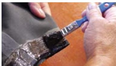
To facilitate the gluing process you might need to fold back the arms of your drysuit for easier access. This action will help in the application of the adhesive in the prescribed area to match the glued surface on the rings. Remember to apply two layers of adhesive and let dry completely between each layer. After the second layer of adhesive has dried you need to invert the arm back to its normal position.
